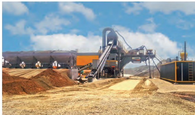
The Linnhoff TSD1500 installed close to the airport produces high-quality asphalt at 90-100 t/hr.
