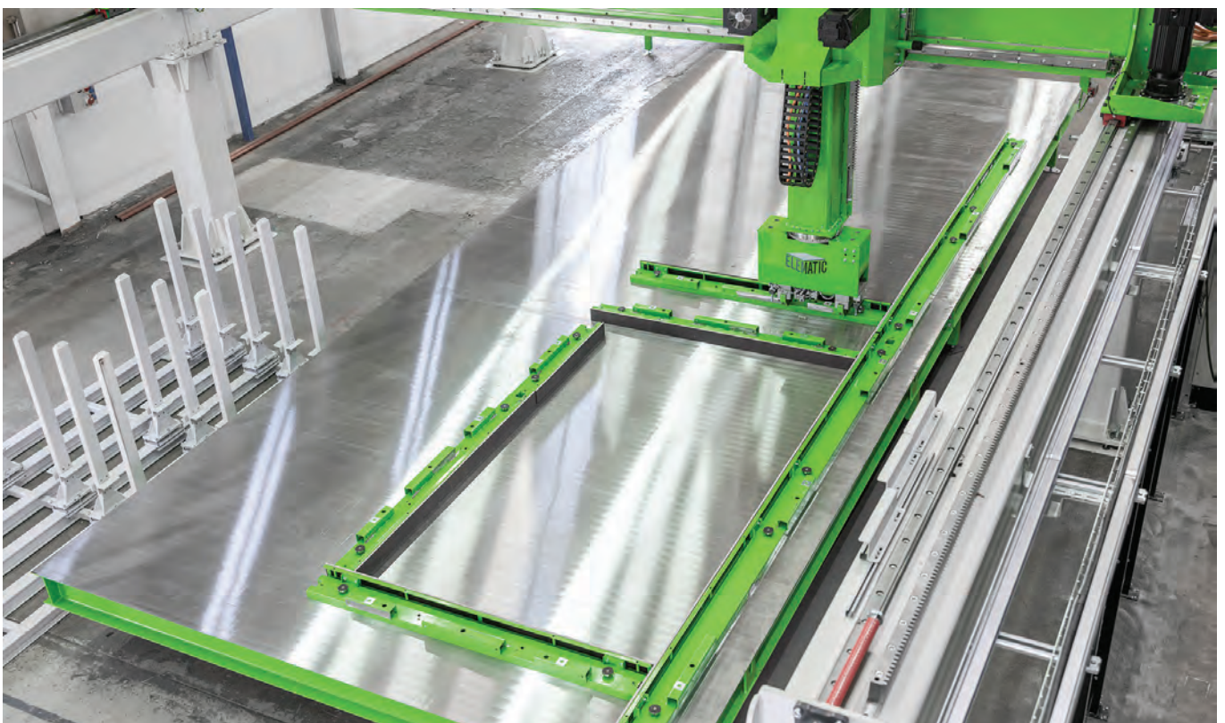
ABOVE AND BELOW: Elematic's new shuttering robot is designed to optimise the automated production of double wall elements. This technology demonstrates the ease and accuracy with which shuttering can be placed on the table, whether it is taken from active or passive storage.
