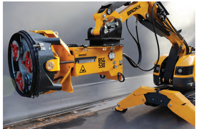
The BSG 530 is fully remote-controlled through the Brokk control box, making it an automated method of stripping plaster, contaminated material, tile adhesive and paint from walls, ceilings and floors.
