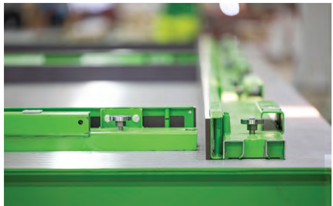
TOP AND ABOVE: Incorporating the latest movement control system for improved controllability and efficiency, the robot is able to rapidly move the shutters, before placing them with pinpoint accuracy, to ensure superbly straight-edged wall panels with sharp 90° corners.
