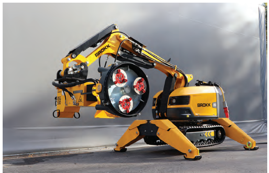
The BSG 530 is compatible with the Brokk 170, Brokk 200 and Brokk 300 demolition robots. Together they can remove material up to 10 times faster than handheld methods.
