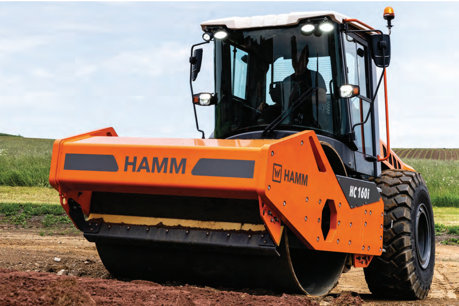
Large slope angles and powerful drives ensure that the new Hamm HC series rollers achieve excellent compaction on uneven and steep terrain – even on inclines over 60%.
