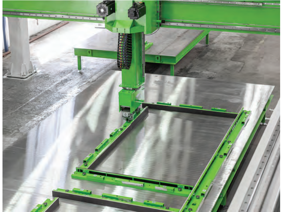
ABOVE AND BELOW: Elematic's new shuttering robot is designed to optimise the automated production of double wall elements. This technology demonstrates the ease and accuracy with which shuttering can be placed on the table, whether it is taken from active or passive storage.
